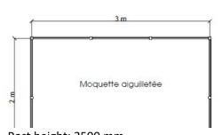
Post height: 2500 mm Length of sleepers: 940 mm Partition panels: 2401 x 952 mm
